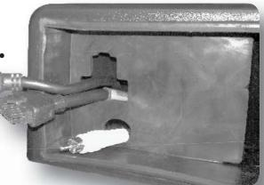
Located on top of the front dash panel is a protruding feature that will fit inside the slotted pod feature. This fit will need to take place prior to snapping in the back half of
