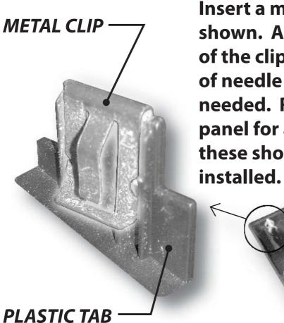
Insert a metal clip over each of the pod tabs as shown. Allow the small "teeth" on both sides of the clip to pierce into the plastic. Use a pair of needle nose pliers to help seat them if needed. Refer to the original panel for a visual of how these should be installed
