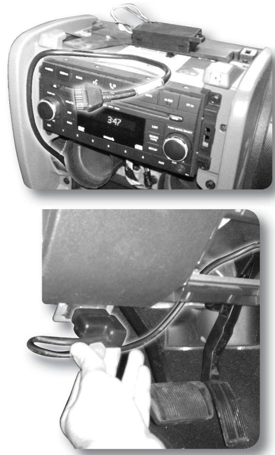
Next, route the cable up and along the side of the radio as shown.
