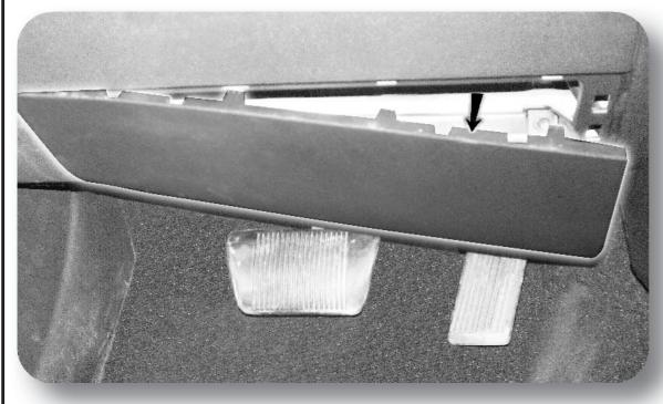
**Remove the lower dash** panel located directly above the foot pedals.
