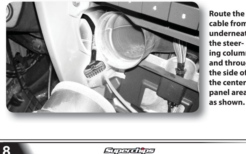
cable from underneath the steering column, and through the side of the center panel area as shown.
