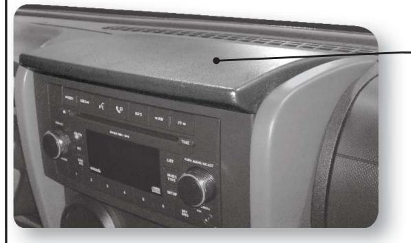
In order to install your new pod, the top dash panel located above the center console will first need to be removed.
