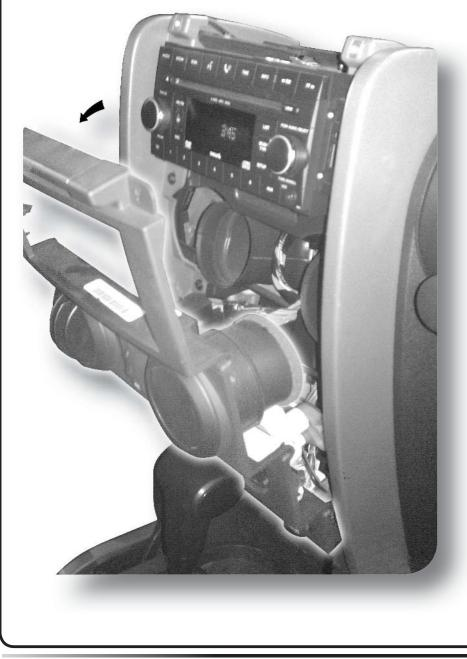
Starting from the top, pull the front panel back and away from the dash.
