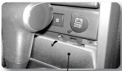
Remove lower panel using the screw driver method as shown in step 1 to expose the screws.
