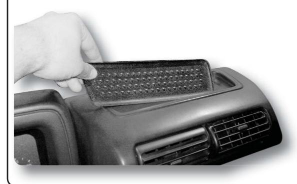
Remove the rubber insert located in the bottom of the dashtop tray. This will need to be removed in order for the pod to be properly fastened into place.
