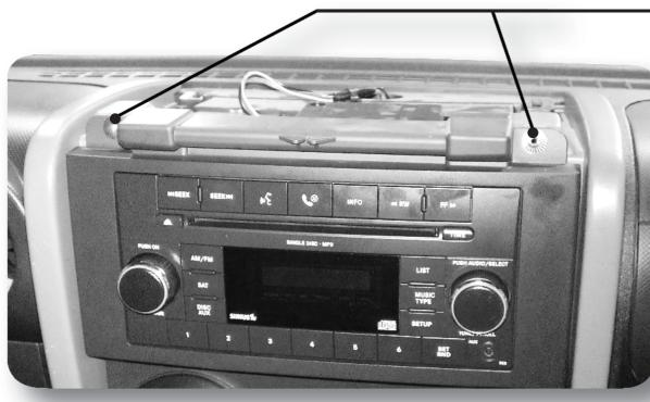
Remove these screws using a 7mm socket or wrench. Set aside.
