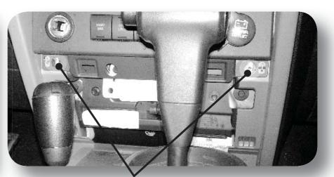
Remove the (2) screws shown using a 7mm socket or wrench.
