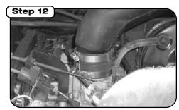
Install intake tube onto throttle body making sure tube is completely resting on throttle body to ensure proper hood clearance. Tighten clamps to
