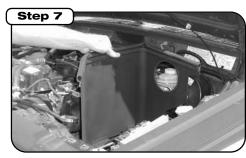
Prior to installing intake housing apply trim seal as shown to housing. Long piece to top edge and short piece lines hole. Place housing and mount. See step 8 for location(s).
