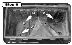
Remove one nut (A) and two bolts (B & C) and lift out bottom of air box.
