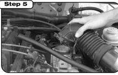
Loosen clamp at throttle body and remove.
