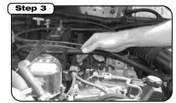
Remove breather tube from valve cover vent.
